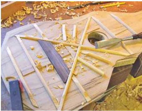
▲ Pic.7 After you've pared down the braces with a chisel, the soundboard is complete
